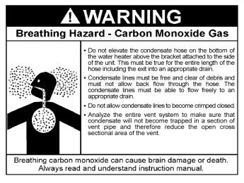
Condensation warning: this water heater is a condensing unit and requires a drain to be located in close proximity to allow condensate to drain safely. The condensate drains from unit at the exhaust elbow located at bottom of unit. Note: it is important that the condensate hose not be elevated above the exhaust elbow, see Figure 11. Condensate build-up will block the exhaust outlet, which will cause improper operation.
